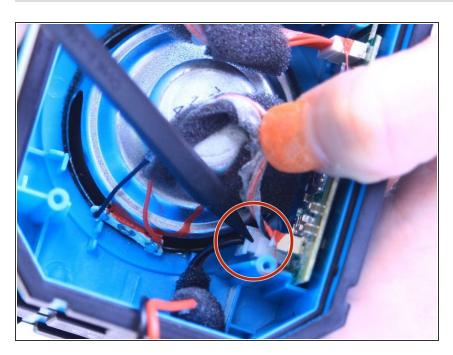
Hold down the small lever on the white, plastic plug attached to the battery wires, and detach the wires from the white, plastic plug outlet on the motherboard.
