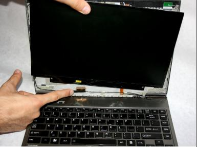
• Disconnect the display cable with your fingers to fully remove the screen from the device.
