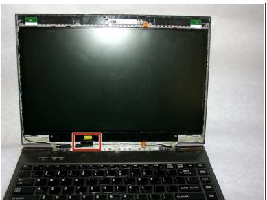
Wedge a blue plastic opening tool between the screen and the frame to free the screen.
