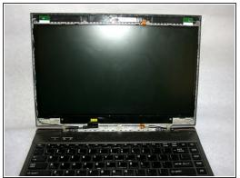
• Use a plastic opening tool to gently pry plastic frame from screen. Detach all housing clips around the perimeter of the screen.
