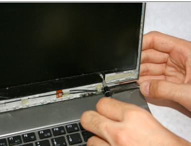
Remove two 3mm screws with a Phillips #000 screwdriver.
