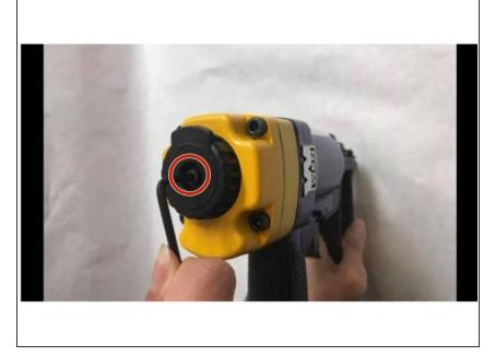
Using a 2mm Allen wrench, remove the Allen screw located on the pressure regulator knob on the back of the brad nailer.
