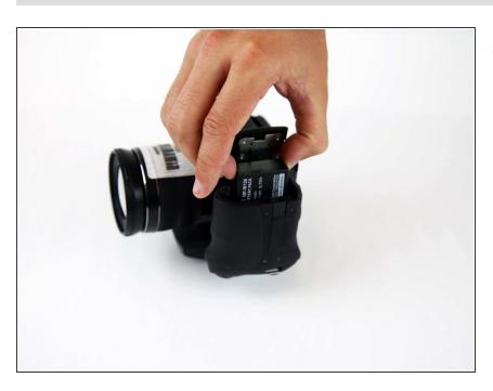
Pull the battery out of the compartment, and replace it with a newly functional battery.
