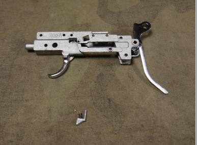
• Now the trigger grouping can be removed from the body and your disassembly is complete.
