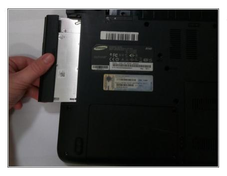
• Slide the optical drive out and remove it from the device.
