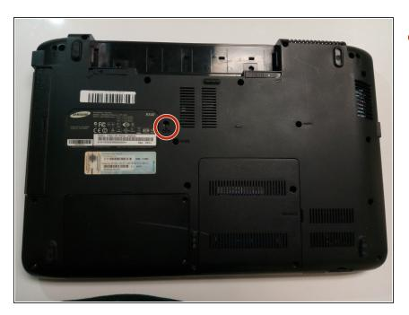
Remove securing screw with the PH0 head.
