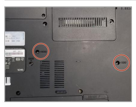
Remove the two Phillips #0 screws labeled KBD.
