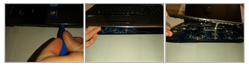
• Pry the front panel away from the base with an Opening Tool.
