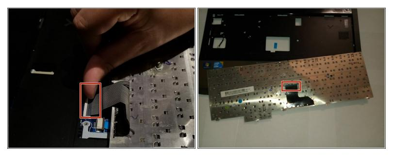
Disconnect the keyboard cable from the motherboard.
