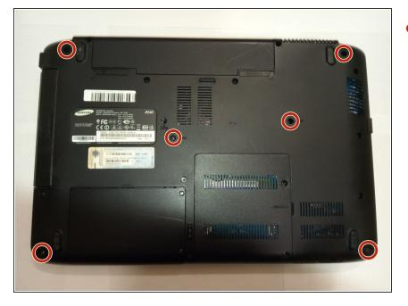
Remove the highlighted screws with a Phillips #0 Screwdriver.
