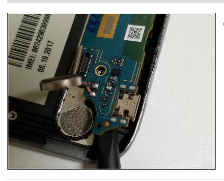
Using the plastic spudger remove the lower logic board because the only thing that is holding it down is glue.
