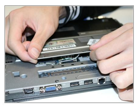
Lift the L-shaped panel by the corners, and set it to the side.
