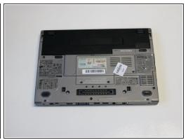
Flip the laptop so that the battery is facing up, and the Dell logo is facing down on the surface the laptop is placed on.
