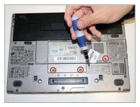
Use a Phillips #00 screwdriver to remove the 3 screws that hold the Lshaped back panel down.
