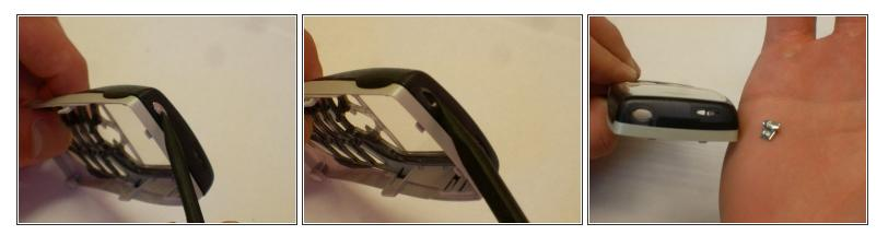
• Use the spudger to push the power button through the casing.
