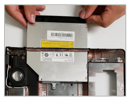
Gently pull the CD drive out of the side of the laptop and remove it from the device.
