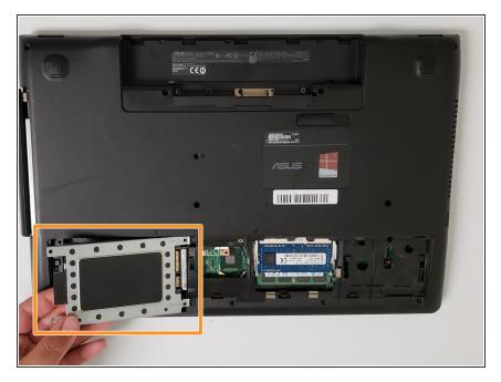
Slide the hard drive to left and remove it from the device.
