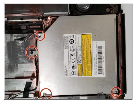
Using a Phillips #0 screwdriver, unscrew the four 4mm screws.
