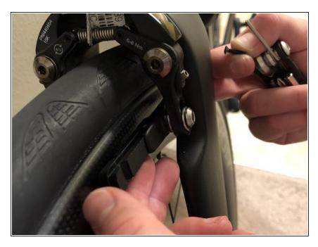
Insert new brake pad into brake shoe.
