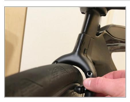
Carefully remove the fairing after the screws are removed.
