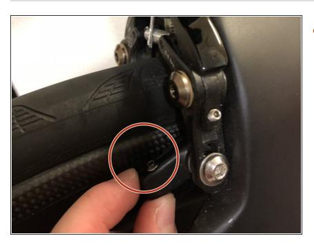
Put the screw back in the brake shoe.
