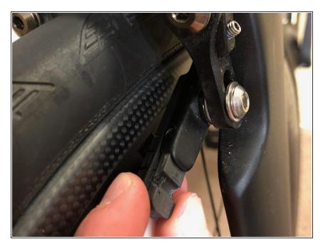
Remove the brake pad from the brake shoe, by carefully sliding it out.
