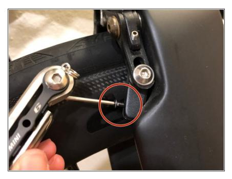
Remove the screw from the brake shoe.
