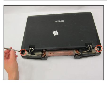
Remove two 5.5 mm Phillips #0 screws on the left and right sides of the device directly behind the screen.
