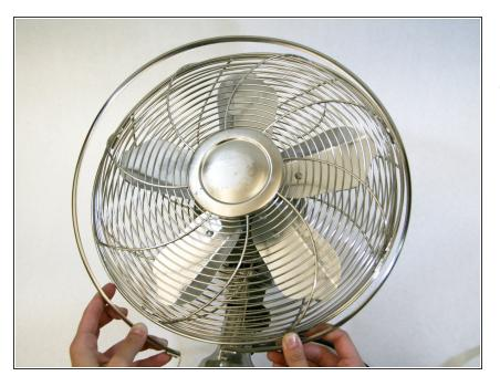
• Remove the ring that runs around the edge of the fan cage.
