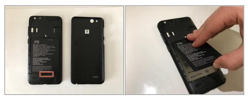
Find the divot near the bottom of the battery and remove the battery from the device.
