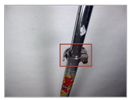
Locate the T-tube clamp. It is in the middle of the steering column.
