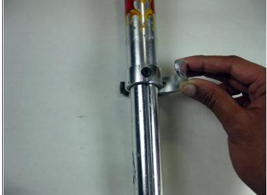
Open the clamp by pulling the lever away from the scooter.
