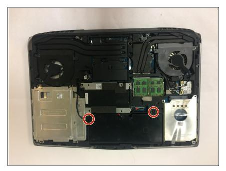
Remove the two 5.5 mm Phillips #0 screws holding the battery in place.
