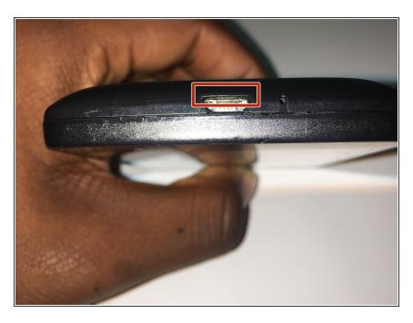
Use a prying tool or a flat head screwdriver to pry the back cover from the device.
