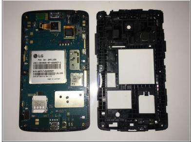
Once you have pried off the back piece, the mother board should be exposed. Set this piece aside for replacement or reassembly. To reassemble your device, follow these instructions in reverse order.
