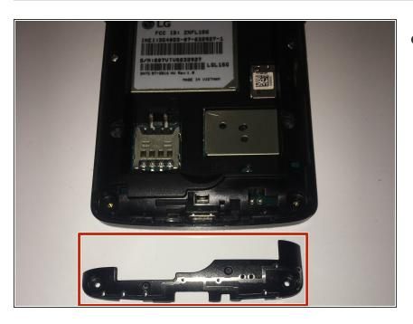
Once both of the screws are out you can easily pop off the bottom piece.
