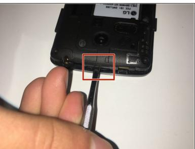
Once you have removed all 6 screws. Gently pry all sides of back plastic piece, starting at the bottom. Once you start on the bottom, it will become easier to pry.
