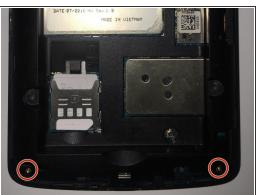
You will be first removing the two lower screws. This is allow you to remove the lower plastic piece.
