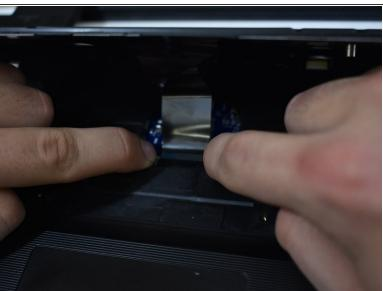
Push the two tan brackets towards the back of the computer, and safely pull out the connector ribbon.
