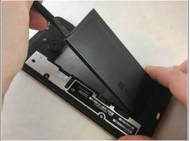
• Lift the battery away from the phone with the flat side of a spudger.
