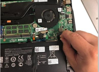
• Disconnect the battery from the motherboard by pulling the black tab attached to the cable.
