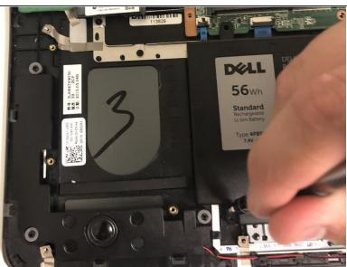
Remove the four 2.5x6mm screws using a Phillips #1 screwdriver.
