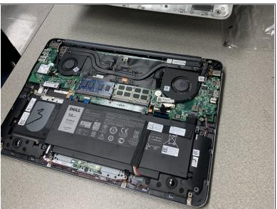
Pry out the back panel using the flat head side of the spudger.
