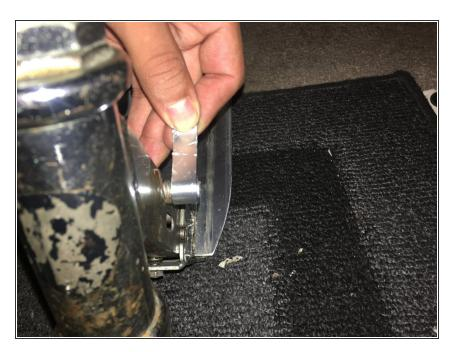
After applying the oil and waiting roughly 5 to 10 minutes you'll pull forward the little lever to fold the scooter
