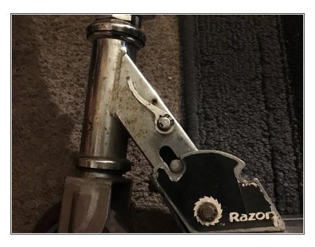
Locate where you'll need to add the oil onto the folding mechanism.
