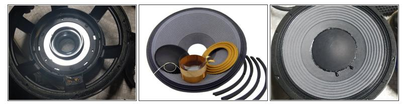
The original coil must have a can placed over it. The suspension must be glued with gorilla glue then the cone. The dust cover needs to be glued in the center of the speaker. The surround then has to be glued around the speakers frame, but carefully as there are screw holes that must be cleared from the surround. Wait for the glue to harden.
