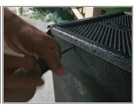
The frame of the speaker needs to be unscrewed carefully and the frame need to be carefully taken off. This is to not damage the frame itself.
