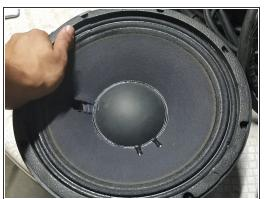
• The damaged speaker needs to be unscrewed from the cabinet. Then once it is unscrewed, left it up carefully but not too high as it is connected to the amp. Carefully disconnected the cables from the speaker and place the speaker on top of a table.
