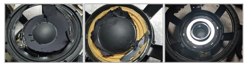
The cone, dust cone, gasket, suspension and surround have to be taken off by cutting it and slicing it out with a box cutter or exacto knife.
