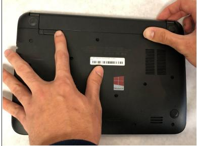
Push slider on left-hand side of device into unlocked position. This slider is not spring loaded so it should stay in position afterwards.
