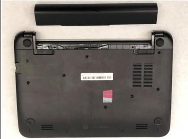
Battery should easily separate from main device.
