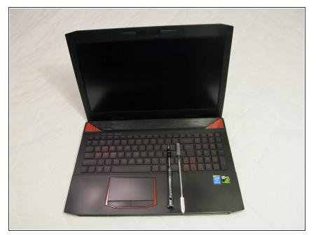
To replace the screen you will need a screwdriver (a size zero was used in this guide), and a tool that can be used to pry off the screen covering (a spudger was used in this guide).
