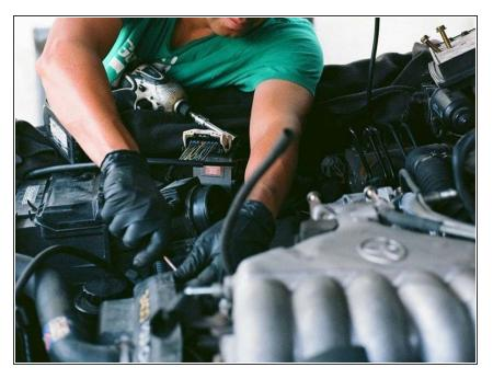
Check your Chevy's battery, the cables, and terminals for any breaks or false connections.
