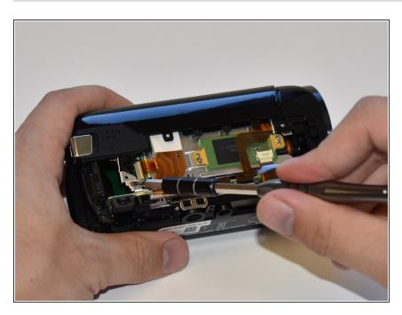
Remove the 4mm Phillips #000 screw that was exposed after taking off the side panel.
