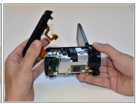
Grasp the top of the camera and pull straight up to remove the top panel.
