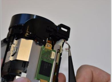
Disconnect the small bundled cable connector on the side of the lens cover by pulling it straight out.
