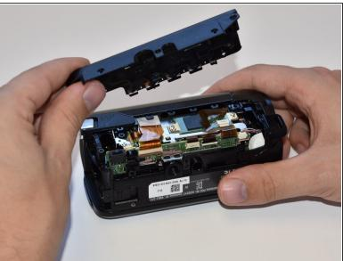
Remove the panel opposite the display by pulling up perpendicular to the side.
