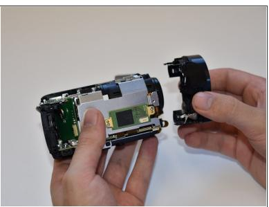
Remove the lens cover by pulling straight away from the body.
