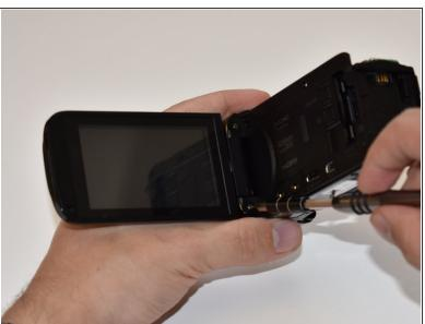
Remove the two 5mm Phillips #000 screws near the display panel.
