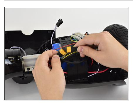
Pull and disconnect the cable connector that is connected to the battery.
