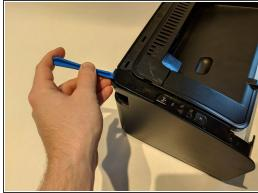
• Using the plastic spudger, remove the button housing from the top left of printer.
