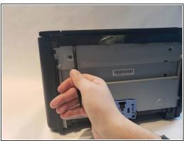
Flip printer on it's back. Using the plastic spudger, pry off front panel. There will be two main points to focus as shown.
