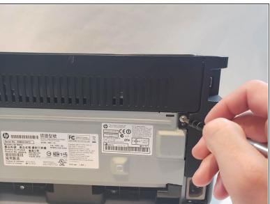
Unscrew the #1 Phillips screw 6mm on the back of the printer.
