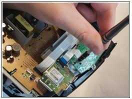
• Remove three #1 Phillips 6mm screws with the #1 Phillips screwdriver.
