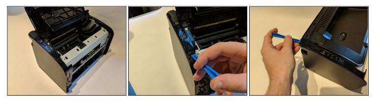
• Using the plastic spudger, remove the button housing from the top left of printer.
