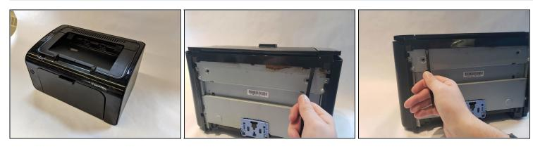
• Flip printer on it's back. Using the plastic spudger, pry off front panel. There will be two main points to focus as shown.
