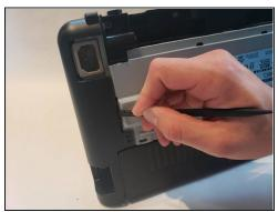
• Use the plastic spudger to remove the side panel. There are three main prying points as shown.
