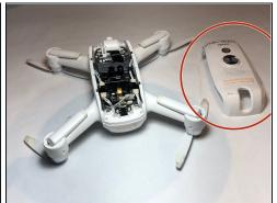
• Grip the cover that covers the rest of the wires, and give it a slight pull to remove it.
