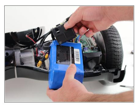
Gently lift the battery harness and remove the battery by lifting the battery and moving it away from the hoverboard.
