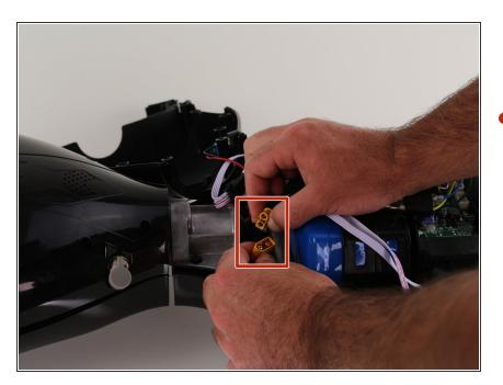
Unplug the battery by pulling gently on both sides of the orange connector.
