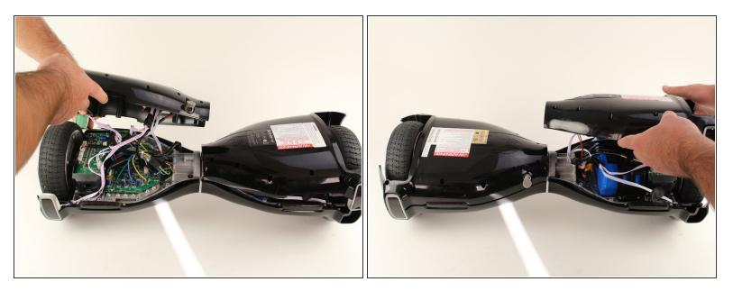
• Lift each side of the bottom shell by pulling up.
