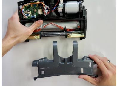
• Using the plastic spudger, pry the back seam of the top component to pop it off the vacuum.
