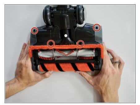
Remove the four 15 mm T10 screws on the underside of the vacuum.
