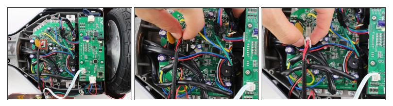
Remove the connector by squeezing the tab and lifting up.
