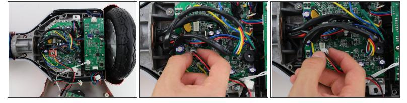
Remove the second connector by squeezing the tab and pulling up.
