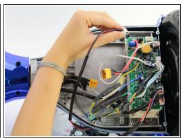
Unplug the red and black charge port wire from the motherboard by squeezing the connector located at the top right of the motherboard and pulling the connector away from the board.
