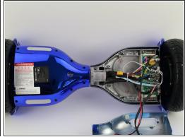
Grip the bottom left panel and lift up to remove.
