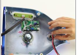
Use an adjustable wrench to loosen the 14 mm nut and lift it off the charge port.
