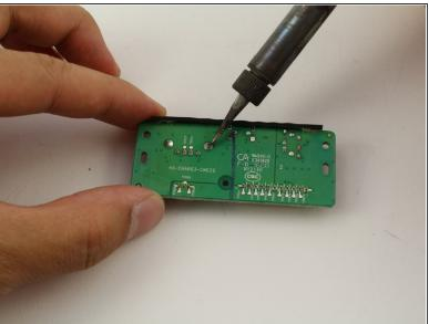
Desolder the USB, MicroUSB, or AUX port off of the circuit board.
