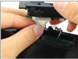
• Disconnect the two bundled cable connector from the port bay.
