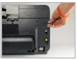
Remove the two 11.6 mm T9 screws from the right side of the back of the printer.
