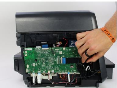
Remove the connectors from the front and sides of the motherboard by pulling straight away from the connection.
