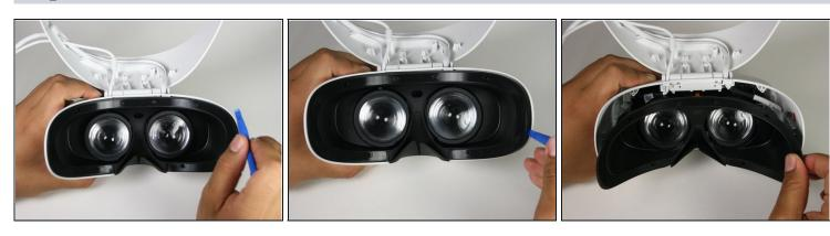
• Remove the cover using one of the plastic opening tools, and then carefully pull it from the casing.
