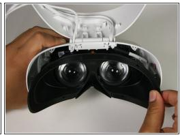
Remove the cover using one of the plastic opening tools, and then carefully pull it from the casing.
