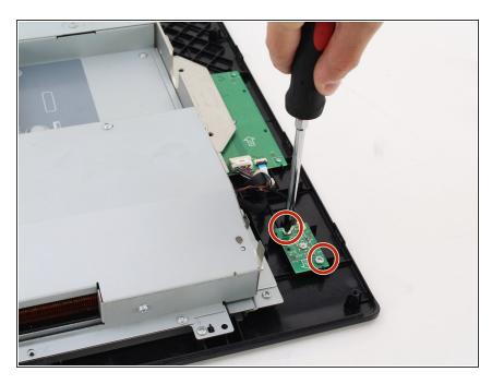
Remove the two 9.5mm Phillips #2 screws by turning the screwdriver counterclockwise.
