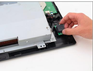
Remove the rubber cover on the power button by lifting up and off.
