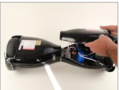
Lift each side of the bottom shell by pulling up.
