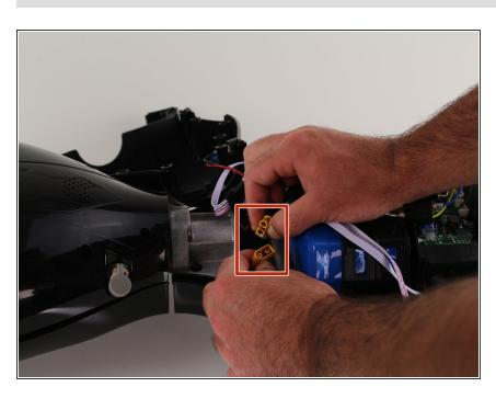
Unplug the battery by pulling gently on both sides of the orange connector. To reassemble your device, follow these instructions in reverse order.
