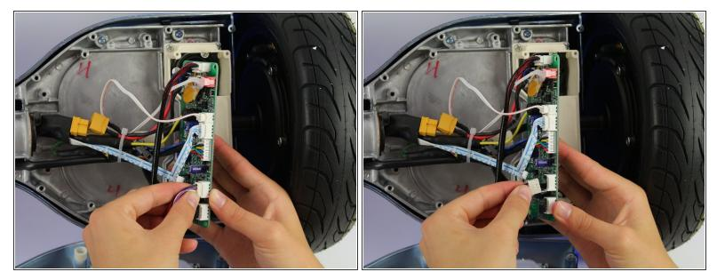
Unplug the light connector by squeezing it and pulling away from the board.
