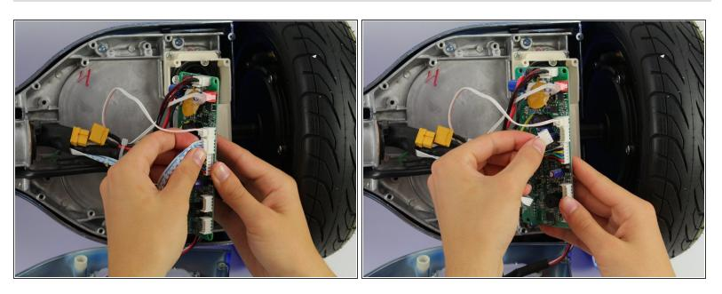
Unplug the blue and white wires by squeezing the connector and pulling away from the board.
