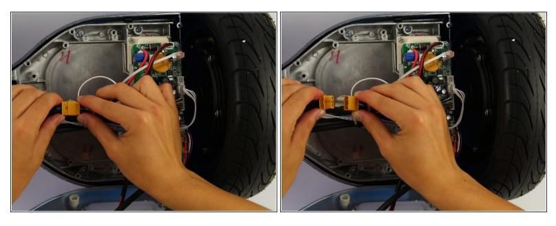
Unplug the battery from the gyroscope by holding the yellow connector and pulling apart.
