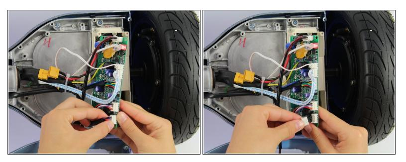
Unplug the bottom right connector by squeezing it and pulling it away from the board.
