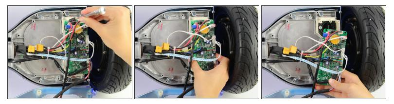
Remove four 12 mm Phillips #1 head screws from the corners of the green gyroscope/motherboard.
