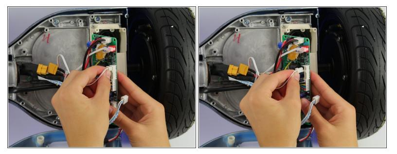
• Unplug the small white connector by squeezing it and pulling away from the board.
