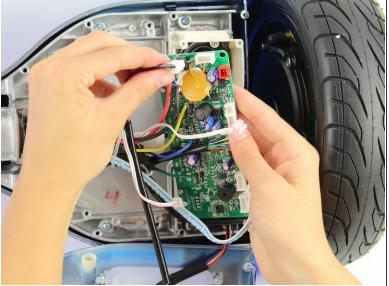
• Unplug the charging cable connector by squeezing it and pulling it away from the board.
