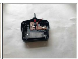
Separate the two halves of the remote controller.
