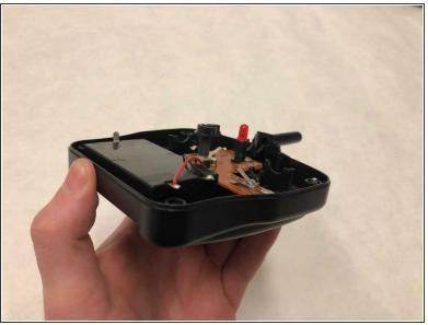
• Lift the metal tab until it is straight and can move through the slot in the battery compartment.
