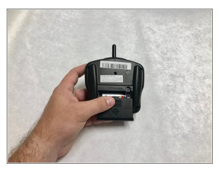
Slide the battery cover off in the direction of the arrow on the cover.
