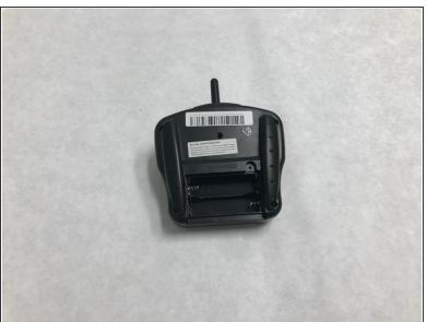
Remove the batteries (2 AA).
