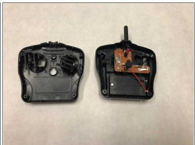
Separate the two halves of the remote controller.
