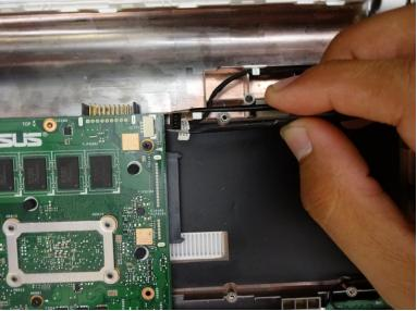
Pull the connector horizontally away from the socket.
