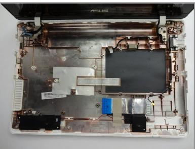
Remove the final piece of the motherboard on the right-hand side of the keyboard shell.
