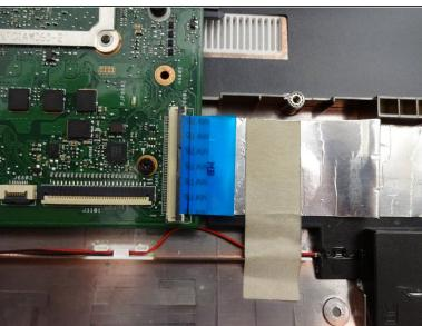
Lift the latch upwards to release the computer ribbon connector.
