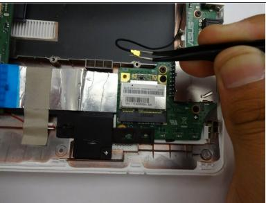
Vertically pull the cable from the head away from the placement.
