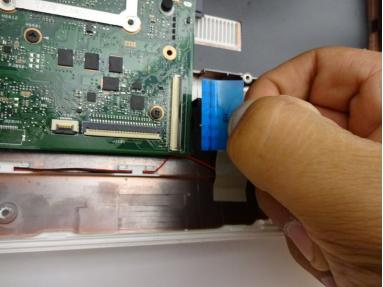
Horizontally pull the computer ribbon cable away from latch.
