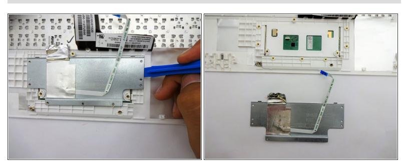
Using a plastic spudger, remove the metal plate.
