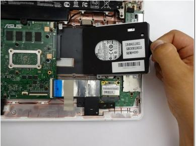
• Remove by sliding hard driving right and away from the computer using the tag on the right side.
