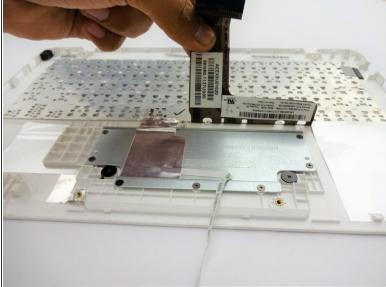
Lift the keyboard connector from the keyboard.
