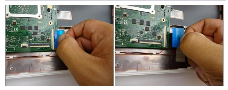
• Horizontally pull the computer ribbon cable away from latch.
