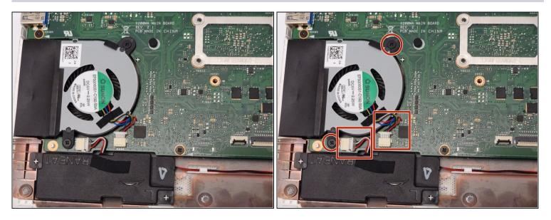
• Locate the fan, two screws and two color coded wires in the bottom left corner of the computer.
