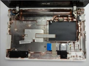
• Remove the final piece of the motherboard on the right-hand side of the keyboard shell.
