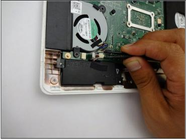
Firmly pull colored wires away from wire slot.
