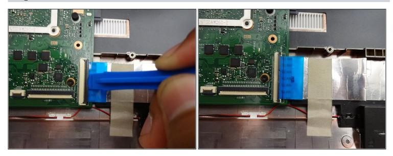
• Lift the latch upwards to release the computer ribbon connector.
