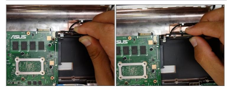
• Pull the connector horizontally away from the socket.
