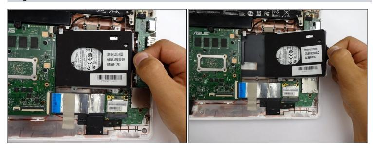
• Remove by sliding hard driving right and away from the computer using the tag on the right side.
