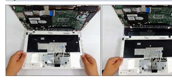
• Now that the keyboard connectors are unplugged, pull the keyboard off and away from the back panel hinges.
