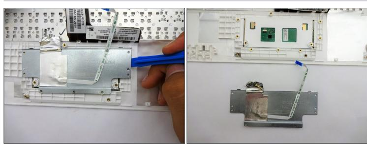
Using a plastic spudger, remove the metal plate.
