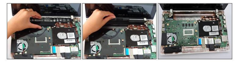
• Gripping the wider left section, lift the battery up and away from computer.
