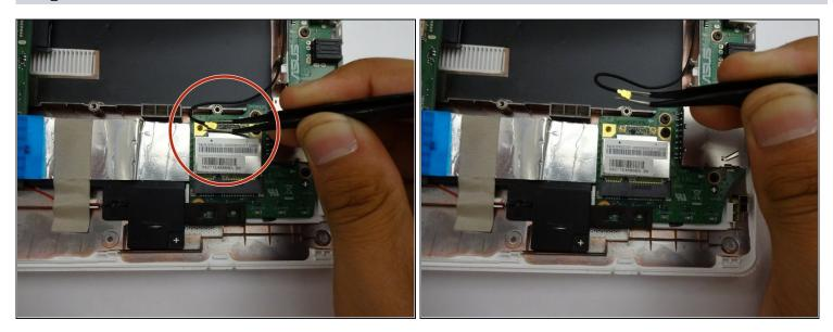
• Vertically pull the cable from the head away from the placement.
