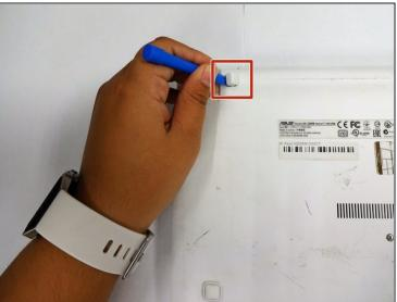
• Using a plastic spudger, remove the two rubber stoppers closest to the hinge to reveal the screws underneath.
