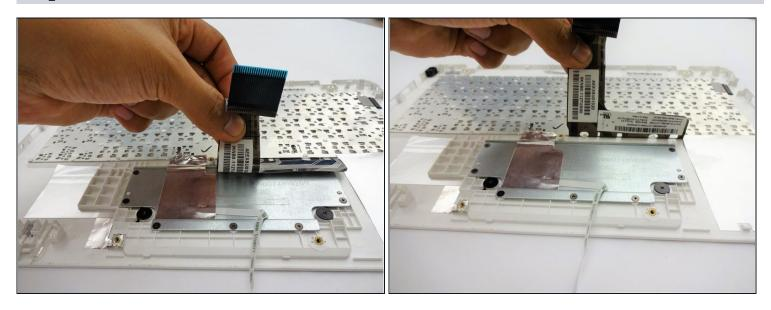
• Lift the keyboard connector from the keyboard.
