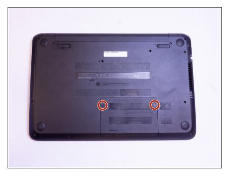
Use a Phillips #0 screwdriver to unscrew the two 2mm RAM shield screws from the bottom of the laptop.
