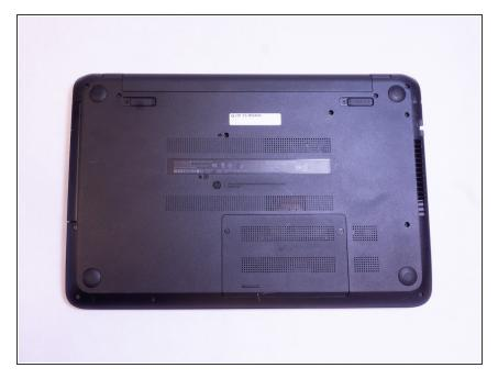
Flip laptop over to the back, so that the stickers are showing and the RAM panel is facing up.
