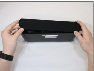
Remove front panel by forcefully placing the flat edge of the spudger in between panel and plastic.
