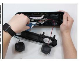
Cut zip-ties wrapped around red and green wires using scissors or pliers.
