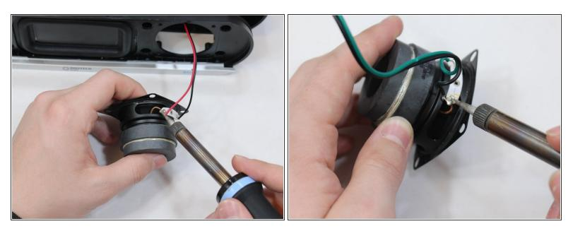
Remove green (left) and red (right) wired connection to speaker bulb using soldering station.
