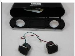
Pull wires out of ports using blunt nose tweezers.
