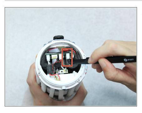
Use the angled tweezers to disconnect the battery from the motherboard. It will take some work to remove this piece.
