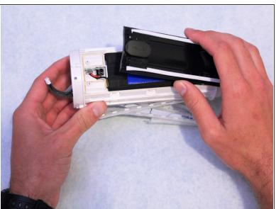
Lift the black centerpiece off with the metal spudger to reveal the battery underneath.
