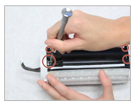
Remove the four 7.9mm Phillips #1 screws from the black centerpiece of the device.
