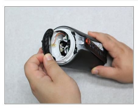
Remove the cover from the end that the ribbon wires are attached to. It should peel off easily.
