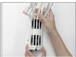
Remove the LED strips from the outside of the white plastic casing.
