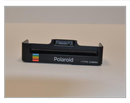
Remove the bottom of the base and piece containing the film door latch.
