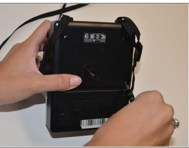
Unscrew the four 5mm screws on the base of the camera using a Phillips #0 screwdriver.
