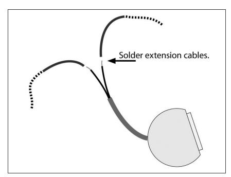
Now solder an extension cable to each of the stripped wires. If you want you can use a red wire for positive (+) and a black wire for negative (-) so you can easily connect the speakers with the amp later.
