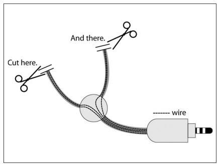
Cut each of the speaker cables. To get the maximum length you can cut the cables near the white "knob" which merges the two cables.
