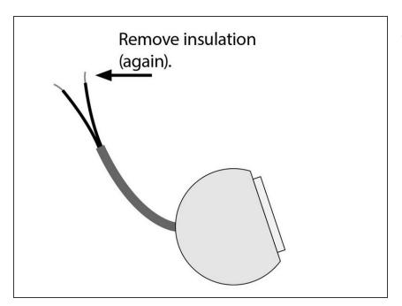
Now also remove the insulation of the small inner wires. Again be careful not to cut the cables as they are very small.
